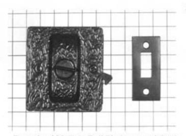
Example of M400 in Dull Black textured finish. All models measure 2-3/4" tall, 2-1/2" across All require minimum door thickness 1-3/8" All require maximum door thickness 1-5/8" Strike measures 1" x 2-1/4"
