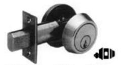
M460 shown in Brass finish with M202 thumbturn. Deadbolt thrown or retracted by key from outside or by thumbturn inside.
